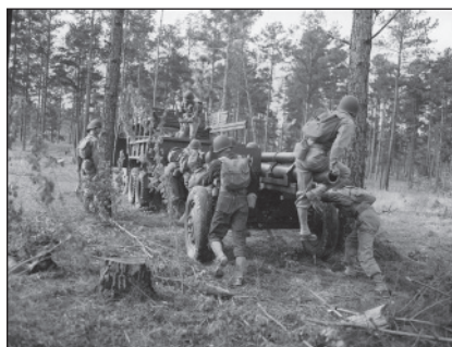
#179 - March order is given and the 105mm howitzer is leveled and backed into the hitch of the 2&1/2 ton prime mover. 26 April 1943, Battery A, 589th FABn, Fort Jackson, SC.
