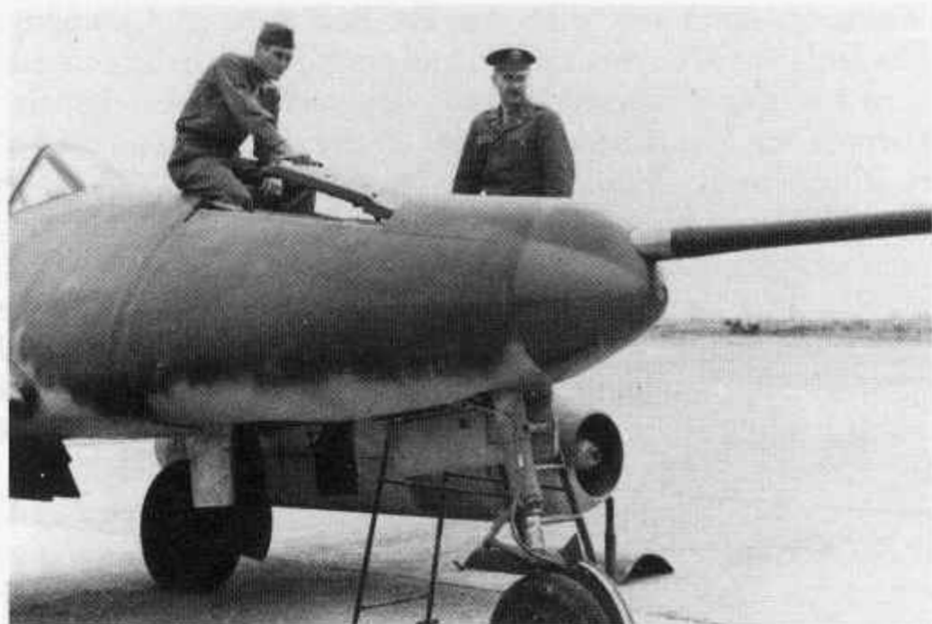
Melun, France, 27 June 1945. TSgt. Ernest C. Parker lifting breech cover of 50mm cannon. (Roy Brown Photo, NASM 78-17898)
