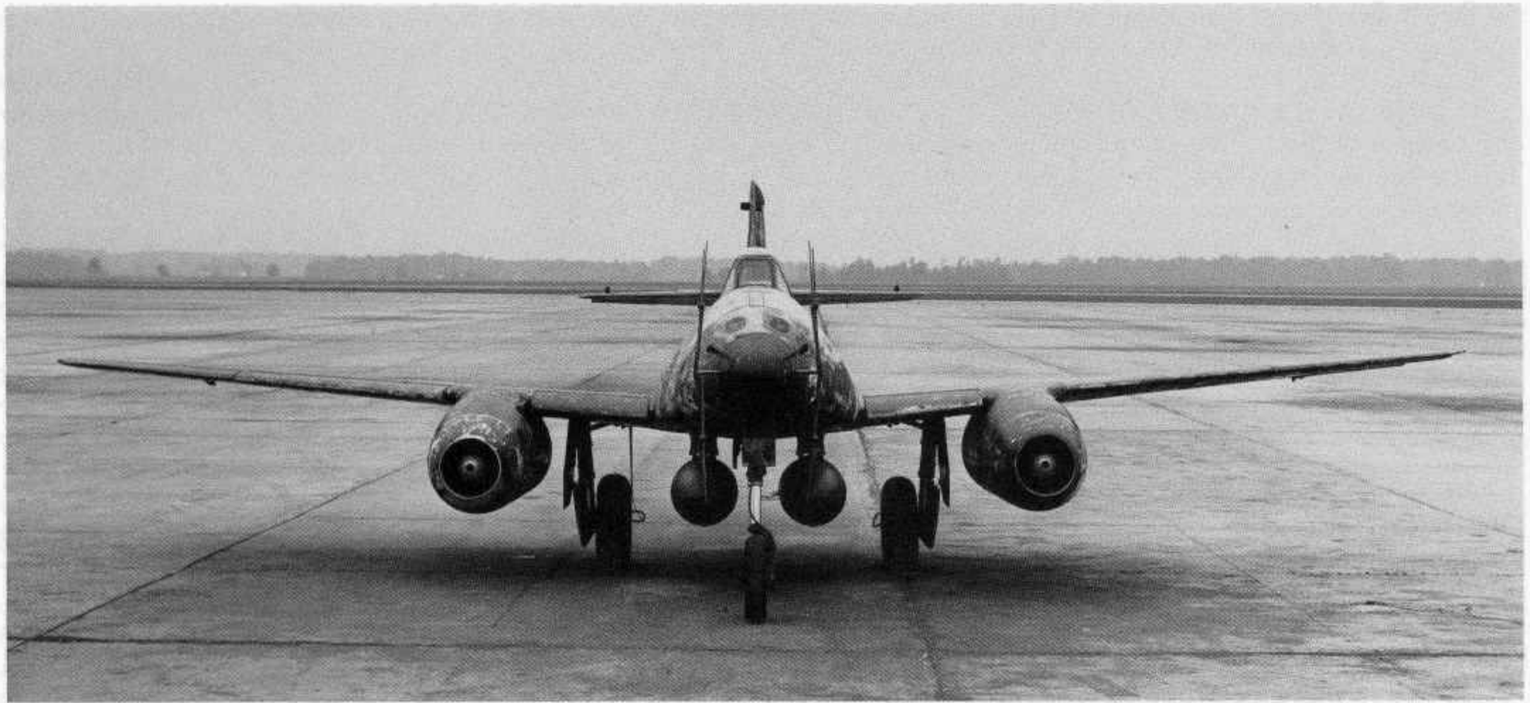
Freeman Field, Indiana, September 1945. Me262B-1a/U1 night fighter variant, FE-610, at Freeman Field. Note radar antenna and external fuel tanks. (H.G. Martin Photo from Robert J. Pickett Collection via Kansas Aeronautical Historical Society)
