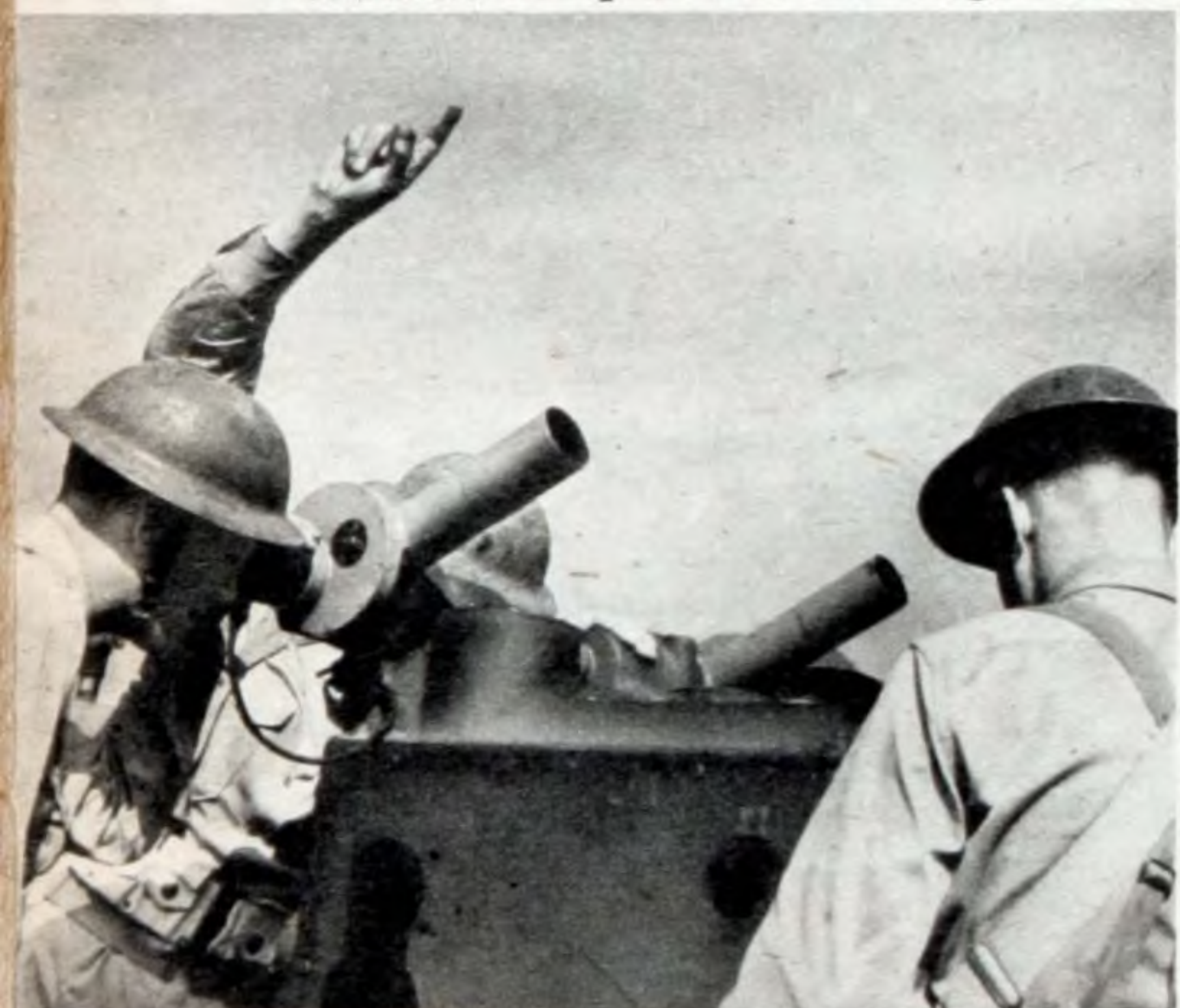
Director. A sensitive precision instrument for use in directing gun to its target.
