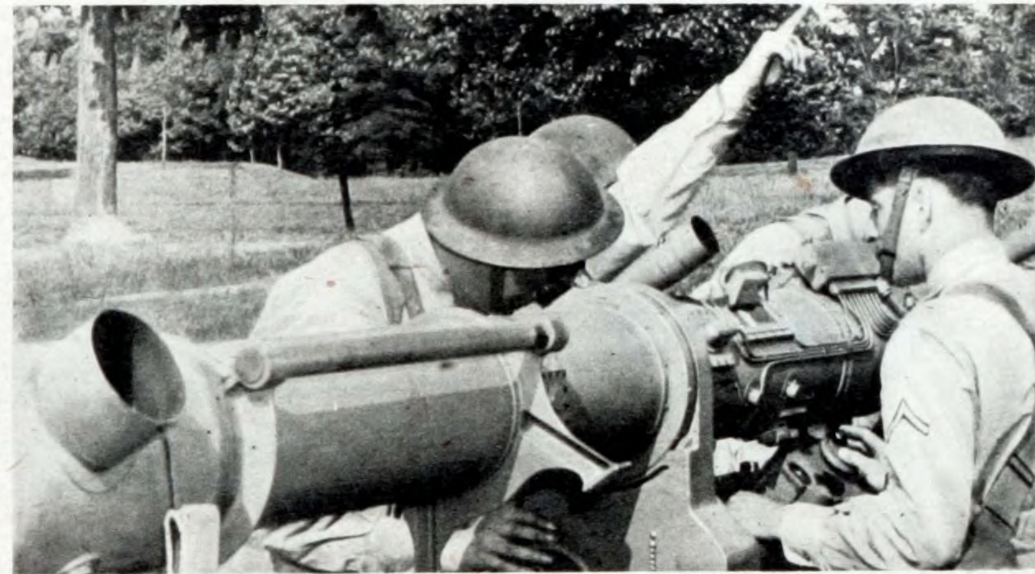
Men on altitude finder get rough data from CP and search skies for raiders. Computed altitude is relayed to "brains" of system, the director.
