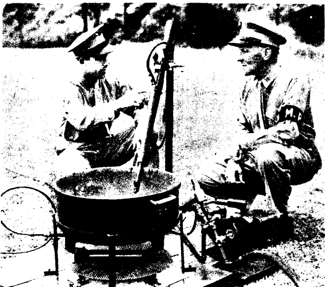
NEW GADGET. Marine Sgt. Sidney J. McMain (left, in photo above) demonstrates his new rifle bath to Capt. Charles Emery at Quantico, Va. Under high pressure, chemically-treated hot soapy water is sprayed through bore by nozzle that fits breech like cartridge (see photo below). It does the whole job in five minutes.
