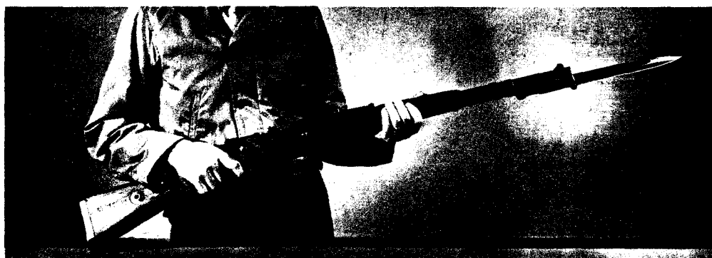
German Model 98K, a short bolt-action Mauser, fires a 7.92-mm bullet (caliber .31).
