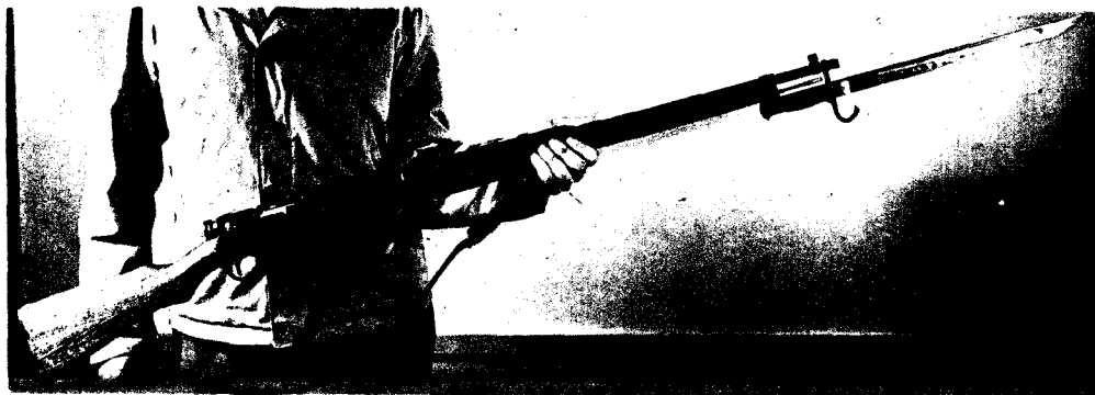
Japanese Arisaka 6.5-mm (caliber .256) doesn't have the stopping power of U. S. rifles.
