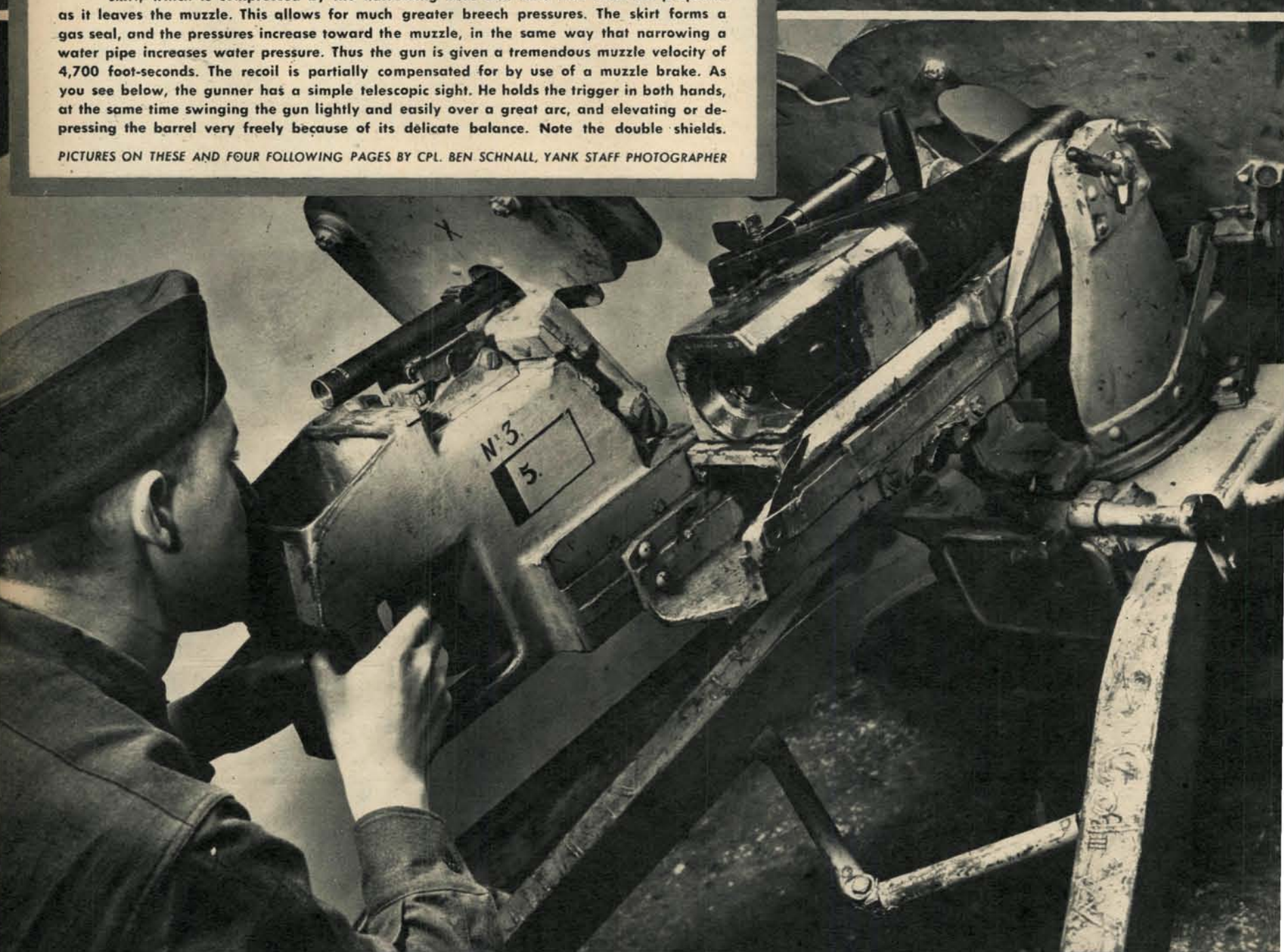
CLOSE-UP OF THE BREECH END OF THE GUERLICH ANTITANK GUN. NOTE THE TELESCOPIC SIGHT AND TRIGGER ARRANGEMENT.
