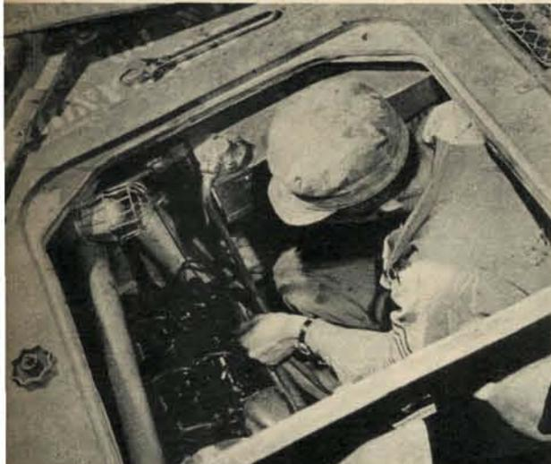
A mechanic at Ordnance Research Center adjusts the valves of the Maybach engine in a PzKW IV.
